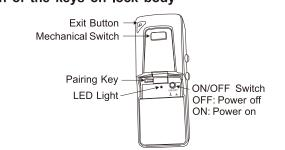
1.Mechanical Switch: Used for installation and equipment trouble, please don't press it often in the normal condition.
