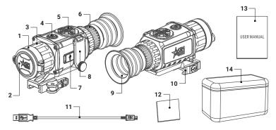
FIGURE 1-1. MAIN PARTS AND COMPONENTS
