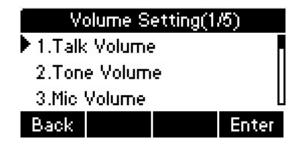
3. User can setup the handset, headset or hand-free volume in different situation. For example, setup the handset talk volume. Enter the Talk Volume interface, choose Handset Volume. Press - or + soft key to adjust. Press Save soft key to save the configuration
