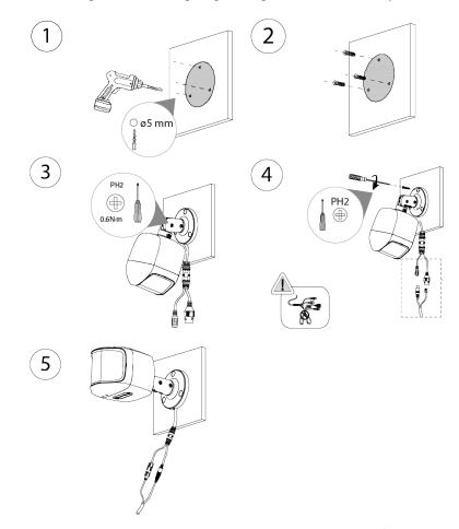
Figure 3-6 Cable going through the mounting surface
