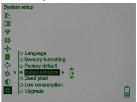
5. For manual dotting selection, short press the knob inward to select this function, the cursor and its X, Y axis coordinates will appear, turn the knob to select "X/Y" coordinates, short press the knob inward to confirm, and turn the knob to change the coordinate value. Short press the knob inward to confirm. After coincident with the dead pixel coordinates, short press the zoom button to do the dotting and save.
