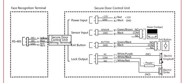
1 The secure door control unit should connect to an external power supply separately. The suggested external power
