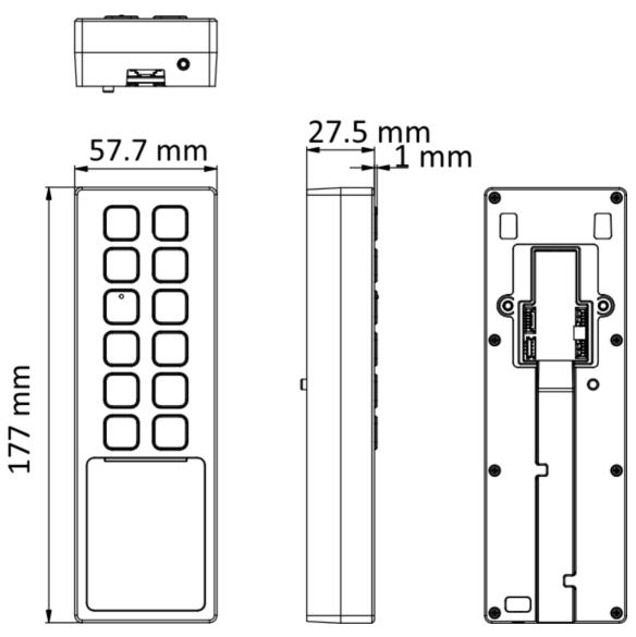
Figure B-1 Dimension of Device (Card Series)
