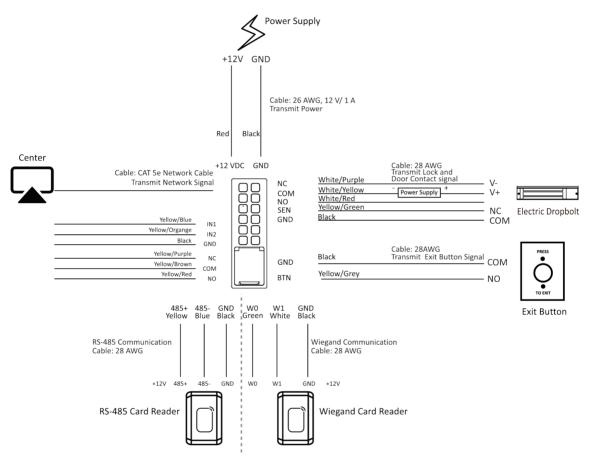
Figure 4-1 External Device Wiring
