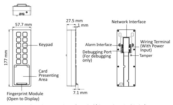
Figure 2-1 Access Control Terminal (Fingerprint + Card Series)
