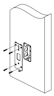
Figure 3-8 Install Mounting Plate
