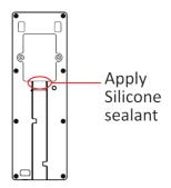
**Figure 3-4 Apply Silicone Sealant**
