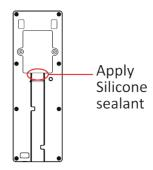
Figure 3-11 Apply Silicone Sealant
