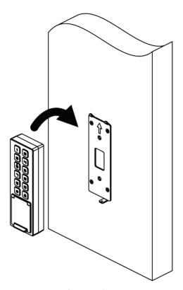
Figure 3-5 Align and Hang Device
