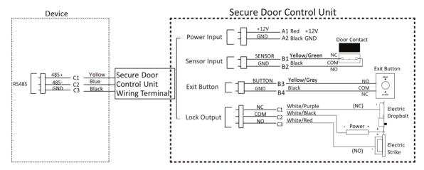
Figure 4-2 Secure Door Control Unit Wiring
