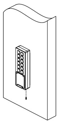
Figure 3-13 Secure Device
