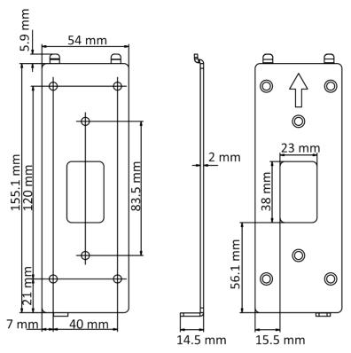
Figure 3-2 Mounting Plate Dimension
