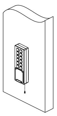
Figure 3-6 Secure Device
