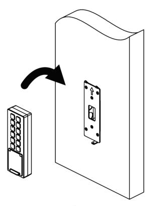
Figure 3-12 Align Device
