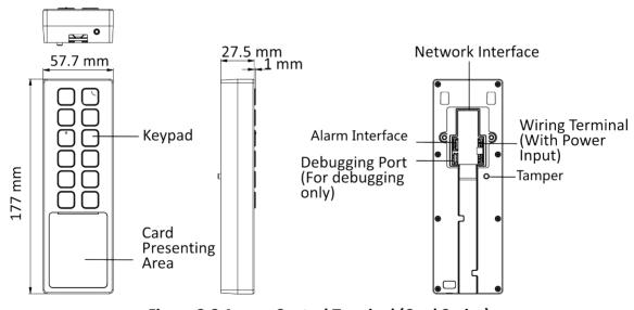
Figure 2-2 Access Control Terminal (Card Series)
