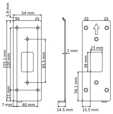
**Figure 3-9 Mounting Plate Dimension**
