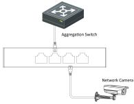
Figure 3-3 RJ45 Port Connection
