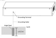
Figure 3-2 Grounding with Angle Steel
