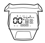
Left direction indicator Right direction indicator High beam indicator READY READY indicator Width lamp indicator Ö Cruise control Electronic control unit
