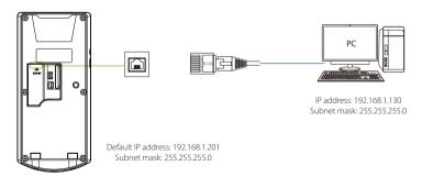
Press **M/OK** to enter the main menu, and select [COMM.] > [Ethernet] > [IP Address], input the IP address and click [OK].
