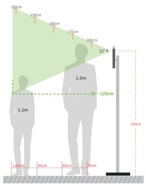
Recommended Installation Height : 150cm Temperature Measurement Distance : 30cm to 120cm
