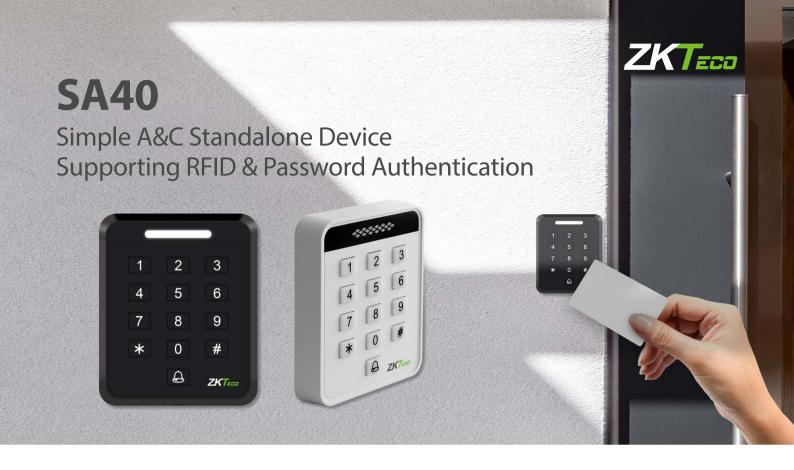
SA40 is a Simple A&C standalone device that supports password and RFID authentication for access control. It supports three different verification modes: password, RFID, password & RFID. Users can be added and deleted in the device, which is very convenient.
