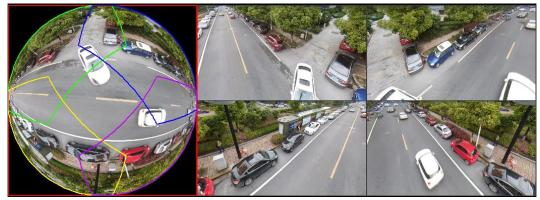
In Figure 4-55, you can adjust the color pane on the left pane or use your mouse to change the position of the small images on the right pane to realize fish eye de-warp.
