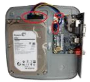
Put the cover back and then fix the screws of the rear panel. The installation is complete. <u>Step 5</u>
