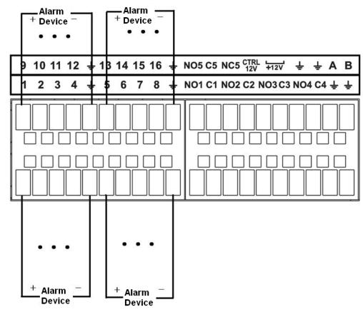
Figure 2-78 Alarm input port
